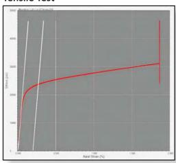
MTESTQuattro® is well suited to perform tensile tests on all types of materials. An example is the control profile for a metals test. The first control segment loads at the prescribed ASTM E8 strain rate through yield. Once the extensometer is frozen and removed from the specimen, MTESTQuattro® automatically switches to crosshead or piston position rate control until specimen failure.
