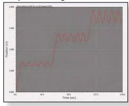
Users can construct complex control profiles with unlimited number of control segments. Ramp, hold, sawtooth and sinewave segments with changes in control channels and rates can be linked together to perform the test you need. Complex profiles can also be repeated to generate more complex cyclic profiles.
