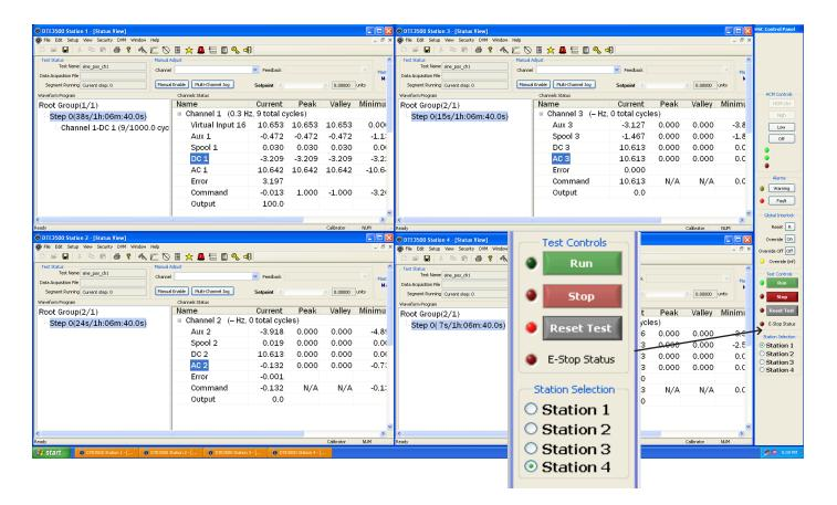
SYSTEM SET-UP is easily accomplished through an intuitive tree structure which can be saved as a configuration allowing easy recall of previous system arrangements.
